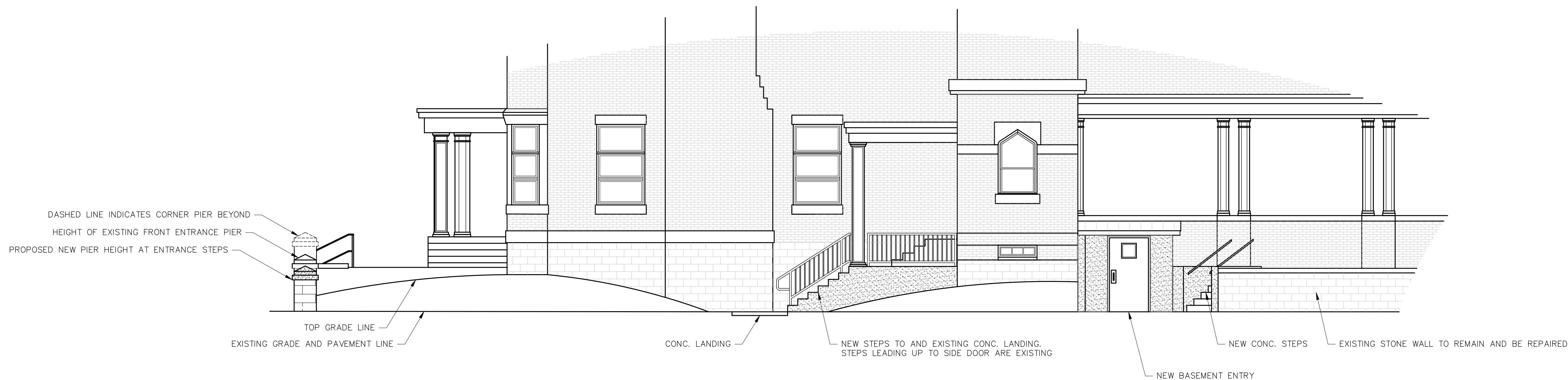
ELEVATION - WEST SIDE OF BUILDING SCALE: 3/16" = 1'-0" 2 SP4
