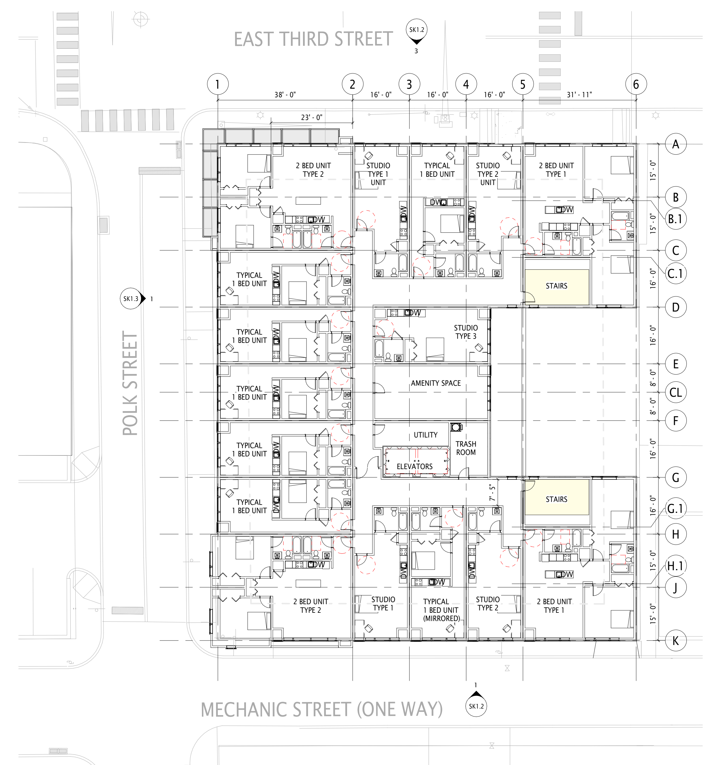
3 TYPICAL FLOOR PLAN (3-7) SK1.1 1/16" = 1'-0"
