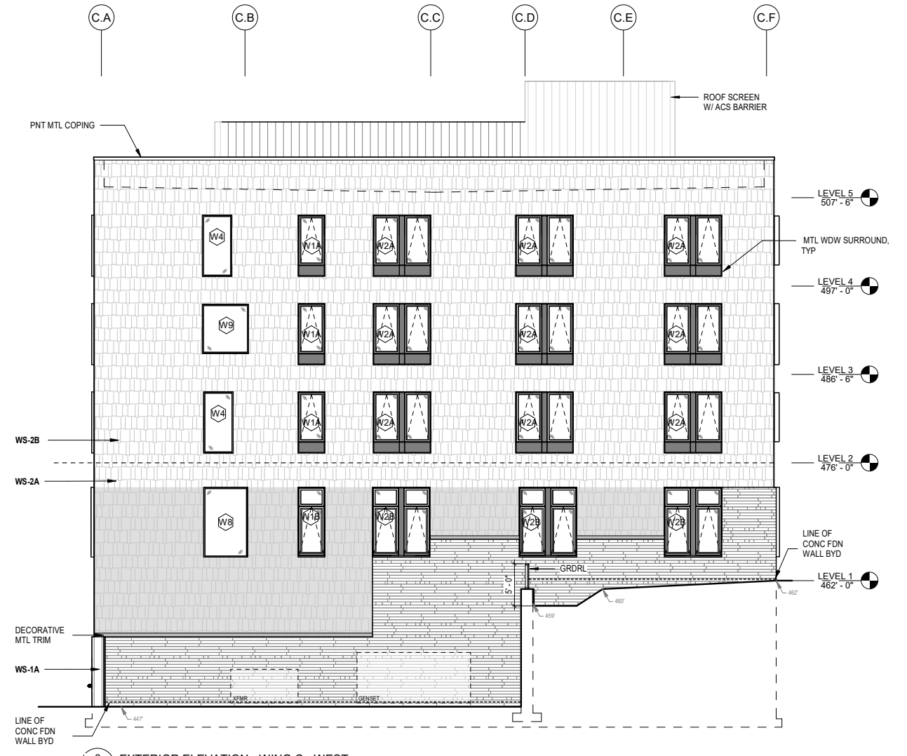
2 EXTERIOR ELEVATION - WING C - WEST A312 1/16" = 1'-0"
