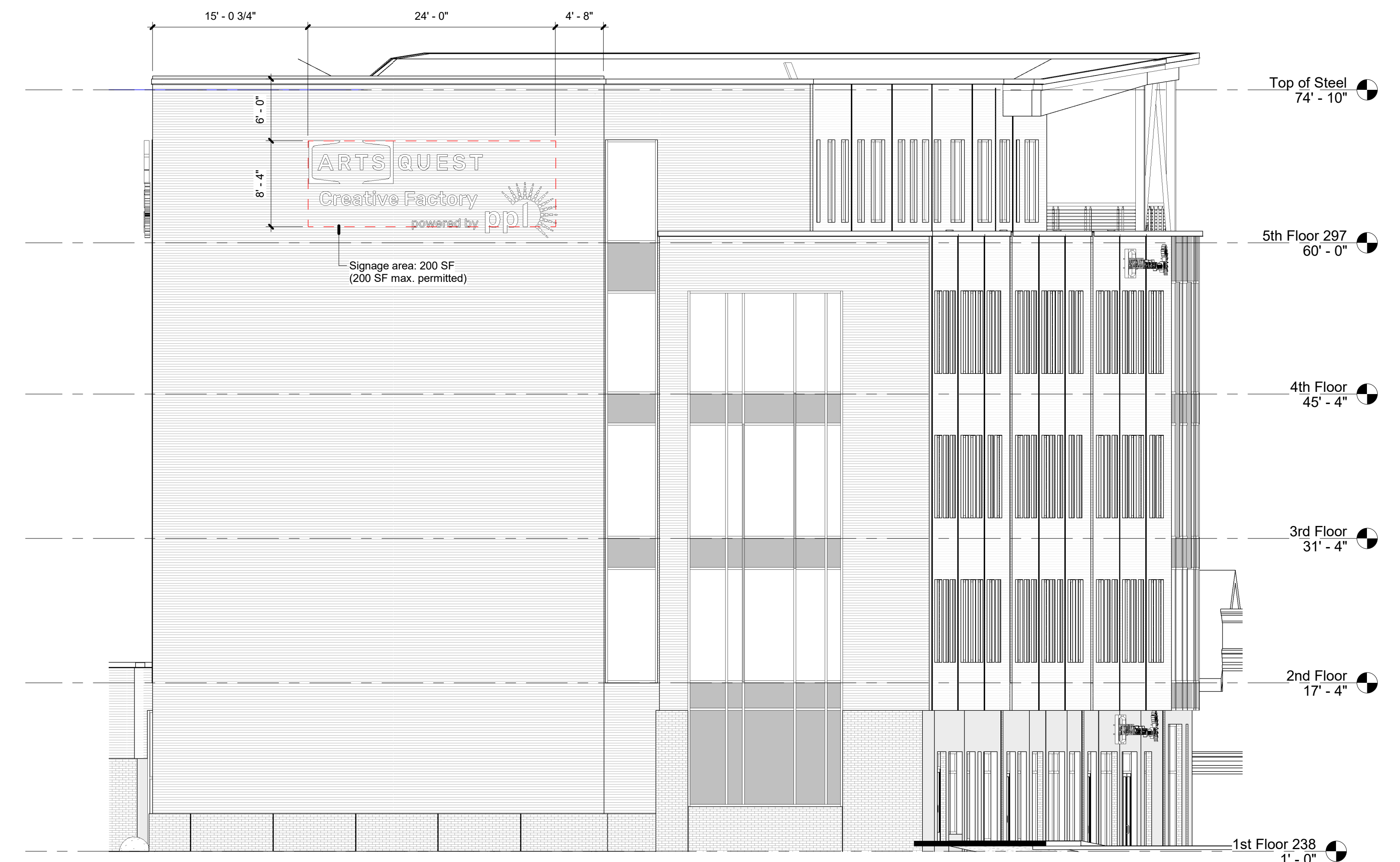
3 West Elevation - HCC Signage 1/8" = 1'-0"
