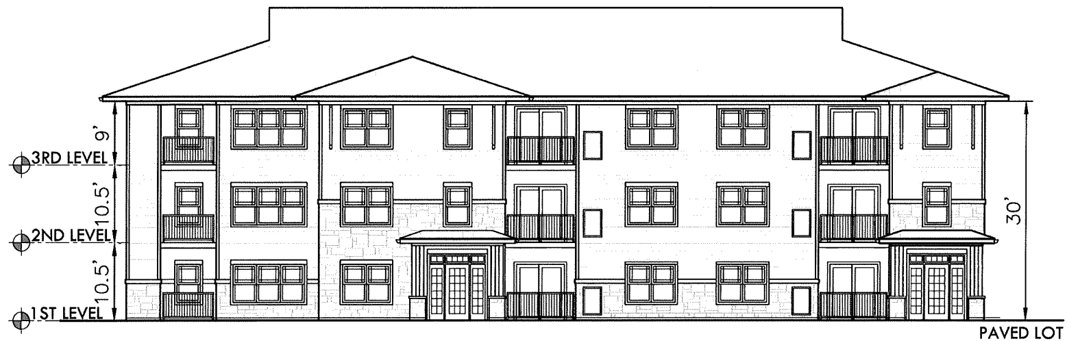
FRONT/CLERMONT ST ELEVATION SCALE: 1/16"=10'-0"
