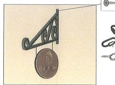
Scroll Bracket with Screws Mounted to Buildina Hang Sign with Eye Bolts and Link Clips
