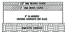
PARKING LOT PAVING DETAIL NOT TO SCALE
