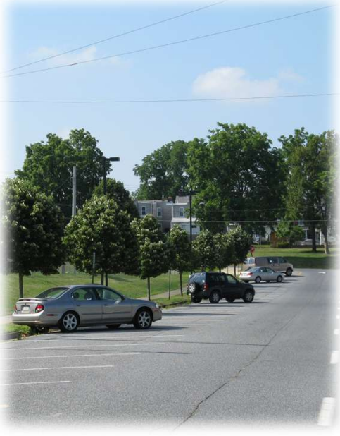
Back-in angle parking can be used to provide more on-street parking and reduce vehicle speeds.
