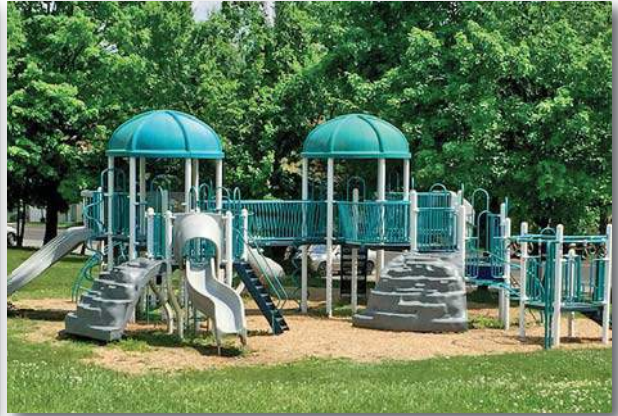
New Component Play Area. Minimal Fall Zones, ADA access not provided, although transfer station is present
