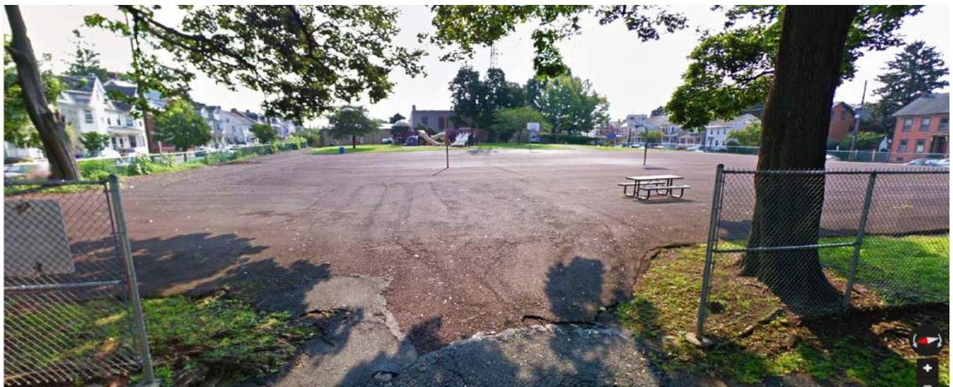
Entrance from Penn Alley for maintenance. Slope of this ramped entry into park does not meet ADA criteria. Walls on North and Garrison Street sides prevent handicapped access.
